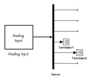
Depending on the board and the number of channels used, I/O conversion time can affect the maximum sample rate that can be achieved on your system. Rather than converting unused channels, specify only the set of channels that your model actually requires.
